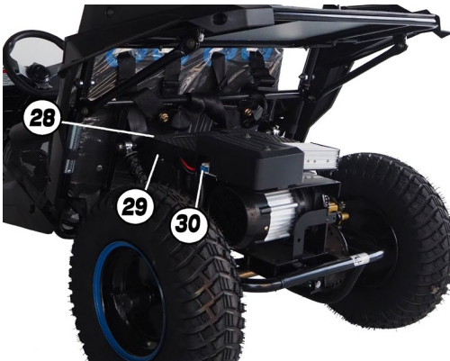
Controller & air break switch box
